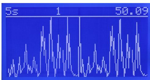
Figure 4: Large Pulse Display permits failing bag rows to be identified during bag cleaning (see FDM, right)
