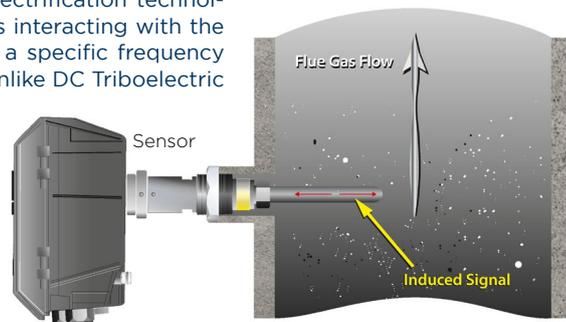
Figure 1: Principle of Operation - *ElectroDynamic™* sensors
