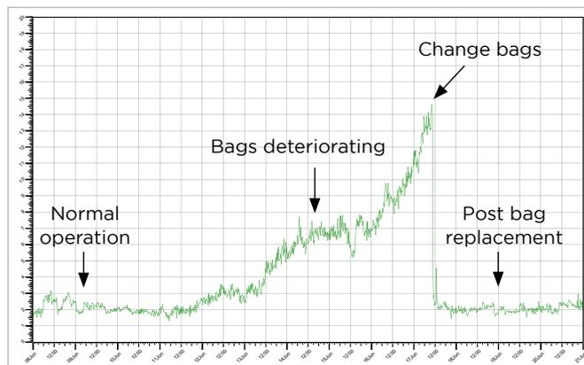
Figure 2: Cleaning pulses highlighting broken and leaking bags (source: PC-ME DUST TOOLS software)
