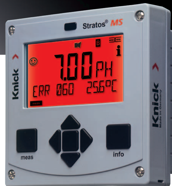
Red flashing display: Alarm, error
