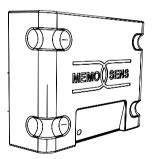
The MemoLink measures 97 x 78 x 38 mm. Thanks to its non-slip rubber feet, it can be conveniently placed on a laboratory bench. The ZU0881 accessory allows wall or post mounting.
