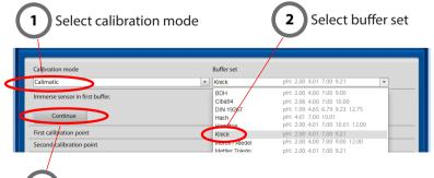
Immerse sensor in first buffer. Select "Continue" to start calibration.
