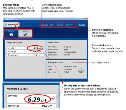
The displayed parameters depend on the process variable.
